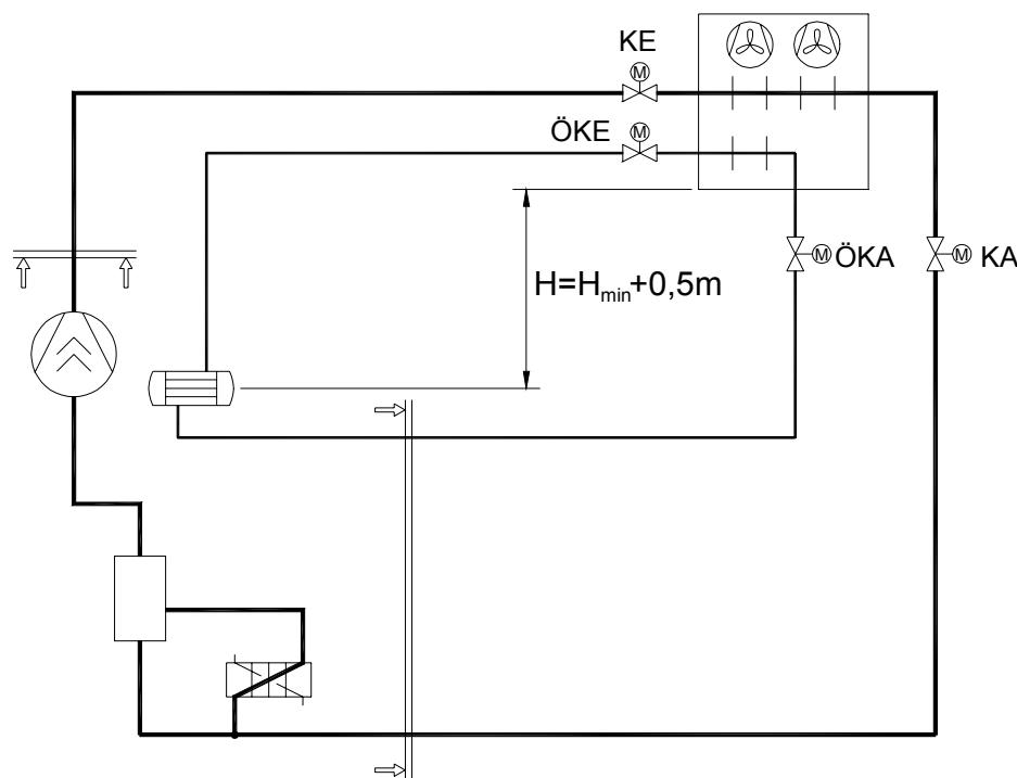
Motor driven valve inlet condenser (KE) and motor driven valve outlet condenser (KA), and additional for suggestion 3 motor driven valve oil cooler inlet (ÖKE) and motor driven valve oil cooler outlet (ÖKA), are controlled depending on compressor operation and ambient outside temperature.
