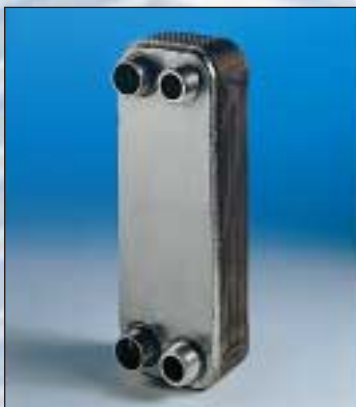
A Nickel brazed PHE for 30 kW flooded ammonia evaporation capacity. Weight: 7,5 kg - Height: 310 mm
