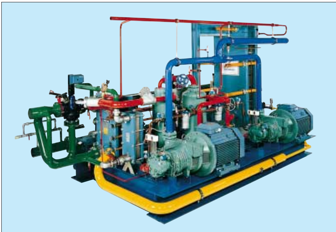
Three PHE models in one NH 3 chiller. M10-BWFDR condenser 480 kW, A15-BWFDR DX evaporator 380 kW, cooling P.G., NB76-FS 46 kW oil cooler. The chiller to cool a fruit storage was built by Firma Stadtegger, Austria.
