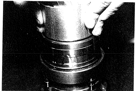
Fig. 101 Installing Piston into Cylinder Sleeve
