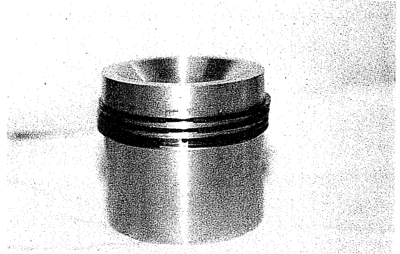
Fig. 90 Improper Arrangement of Piston Rings
