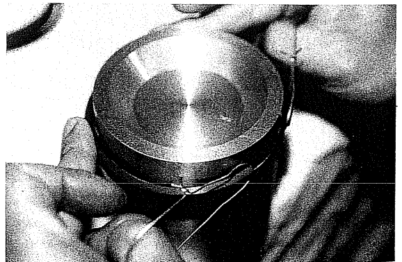
Fig. 46 Removing Piston Ring
