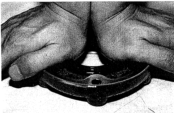
Fig. 83 Reassembly of Floating Seat (Seal Carbon)
