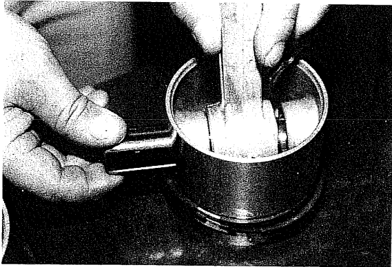
Fig. 92 Mounting Piston Pin
