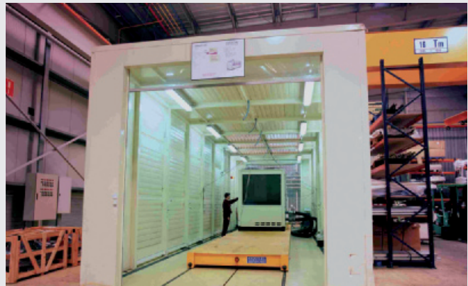
All Samurai chillers are subject to commercial test which simulates real operating conditions.
