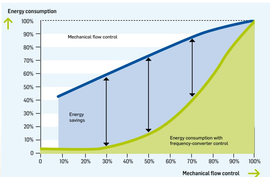
If, for example, the rotation speed of a fan drive ( $M - n_2$ ) is reduced by just **15%**, the power consumption is reduced by as much as **38.5%**. Should, during the entire process, the rotation speed be adjusted to its full potential, the additional outlay for the frequency converter will be recovered in a very short period of time.
