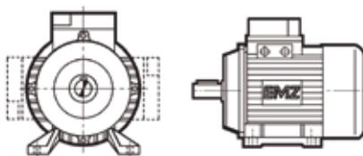
*Removable or "modifiable" motor feet/variable terminal box position*
