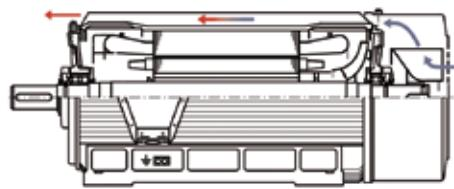
A different type of cooling such as IC416 with external ventilation is also possible upon request.
