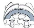
Fig 3 Continued rotation progressively reduces the space occupied by the gas, causing compression.
