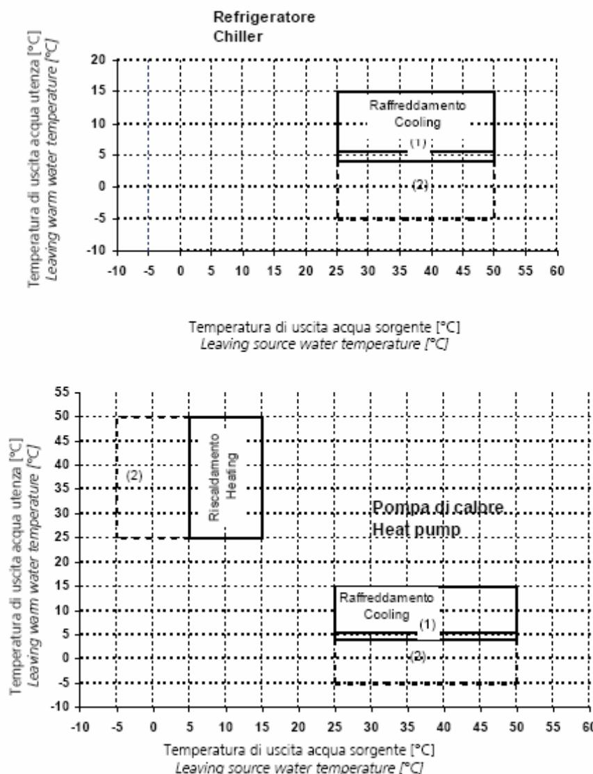
The water temperature rise for all versions must be between 4 °C (min) and 7 °C (max)
