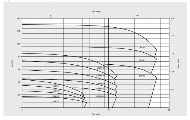
Performance Curve CAM 3600 rpm/60 Hz
