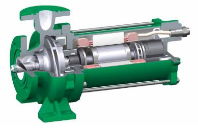
The return of the partial flow to the delivery side ensures that point 3 in the Pressure-Temperature-Diagram (Figure 1) is sufficiently distanced from the boiling-point curve of the diagram. With the CNF model, it is thus possible to pump liquefied petroleum gases with an extremely steep vapour pressure diagram conditions being the same, except for the gas to be pumped.
