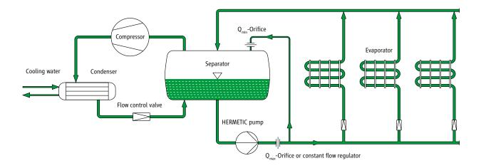
The figure shows the simplified scheme of a large refrigeration plant. The characteristic of this plant is that the refrigerant flows through a central fluid separator and is then conveyed to the evaporators. The resulting vapour and the surplus fluid return back to the separator. Compressor, condenser and flow control are incorporated in a secondary circuit.
