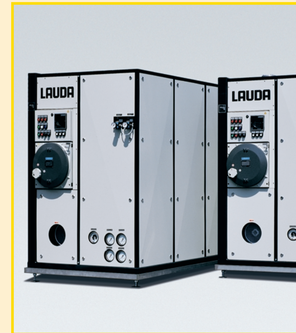
Process cooling unit with water-cooled condenser for installation in hazardous area to control the temperature within a temperature range from -30 up to 150 °C. Cooling capacity 300 kW/0 °C Additional heating steam 500 kW Type SUK 600 W Ex
