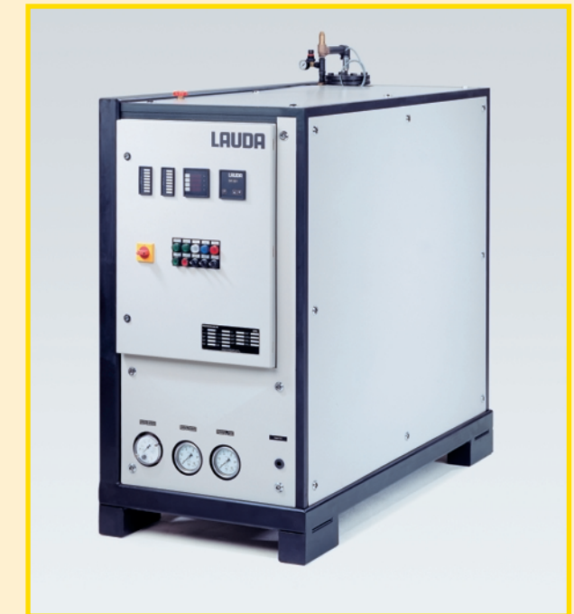
Process cooling unit with water-cooled condenser to control the temperature within a temperature range from -70 up to 150 °C. Cooling capacity 2 kW/-70 °C Additional electric heating 12 kW Type SUK 350 W II
